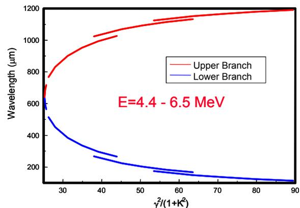
Figure 2: Wavelength range of the THz FEL depending on the energy of the electron beam from the microtron.
