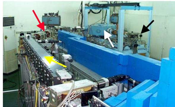
Figure 1: Photograph of a compact terahertz free electron laser driven by a magnetron-based microtron. The length of the undulator is 2 m and a high voltage modulator for RF generator is located under the microtron and RF system.
