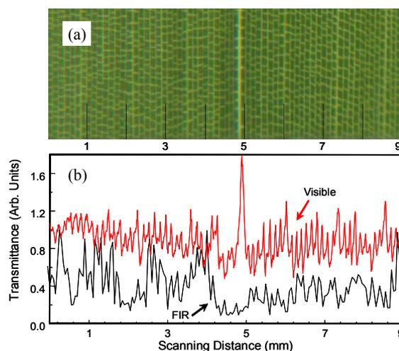
Figure 4: One-dimensional FIR scanning with an aperture of 0.1 mm performed with a bamboo leaf. The result was compared with a scanned intensity profile of the photograph shown in upper part of Fig. 4 (b). The photograph of the leaf is shown in Fig. 4 (a) with the same scale of the scanned profiles in Fig. 4 (b).
