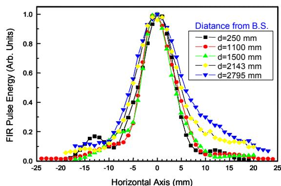
Figure 3: Measured spatial distribution of the FIR radiation at the experimental tables of the facility. The distances noted in the figure are values between the measured points and the beam splitter for pulse energy monitoring.
