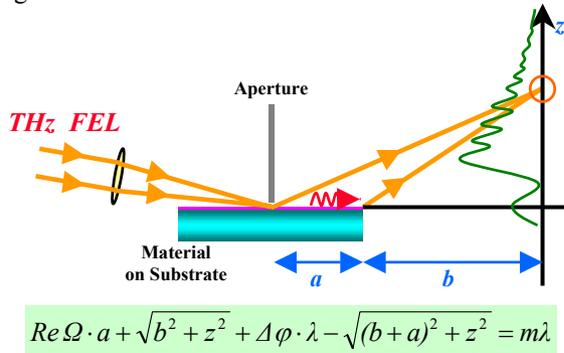
Figure 5: Schematics of thin film SEW measurement.
