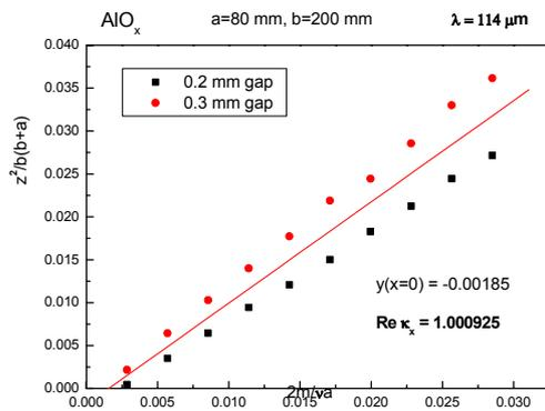
Figure 6: Measured optical constants of AlO<sub>2</sub> thin film having the thickness of 3 nm.
