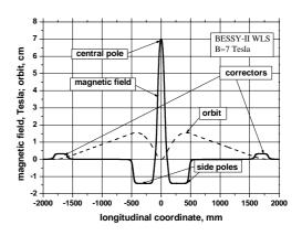
Fig.1: The distribution of magnetic field and electron beam orbit along BAM-WLS straight section
