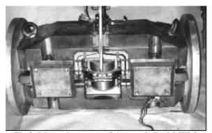
Fig.2: Magnetic system of three-pole BAM-WLS
