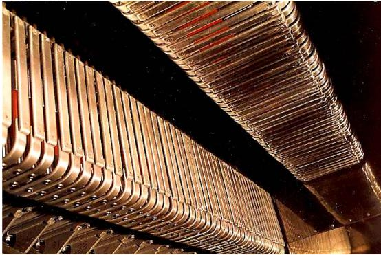
Fig.1. Glass-glaze resistors on the machine
