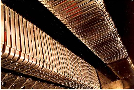
Fig.1. Glass-glaze resistors on the machine
