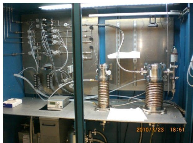
Figure 13: Reactors at Temple University for small size (left) and for 2-inch diameter (right) MgB_2 films.
