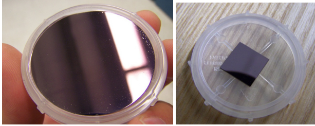
Figure 14: 50.8 mm diameter (left) and 1 cm x 1 cm (right) samples prepared at Temple University using a hybrid physical chemical vapour deposition (HPCVD) technique.
