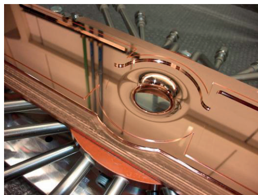
Figure 4: Surface of cell two of the gun before brazing.
