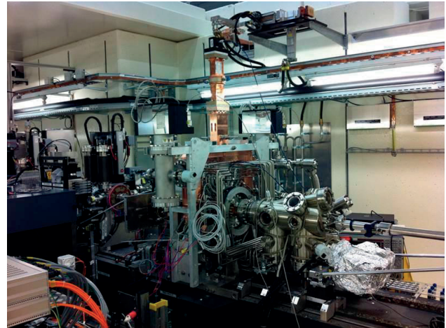
Figure 7: Setup of the RF gun for power testing at the 250 MeV test facility at PSI.
