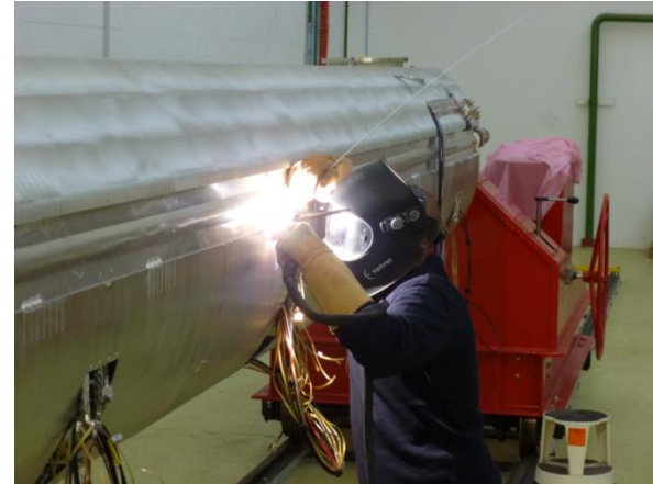
Aluminium thermal shields welding
