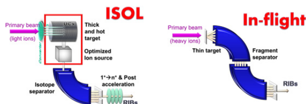
Figure 1: ISOL and In-flight RIB production methods.
