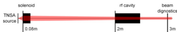
Figure 3: The 15 cm long pulsed solenoid is located 8 cm behind the laser target. It is set to focus 9.6 MeV protons at a 3m distance. At 2m a RF cavity is located followed by a diagnostics box and a magnetic dipole detector.
