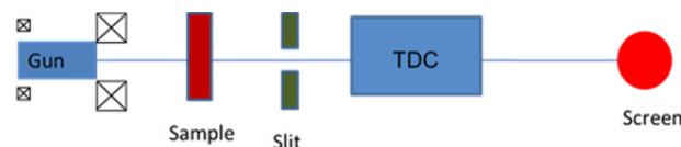
Figure 6: Layout of a “streaking” scheme for diffraction.
