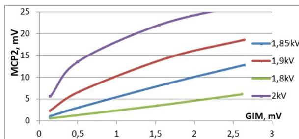
Figure 4: Dependence of MCP2 signal on gas ionization chamber signal at different MCP 2 voltages.
