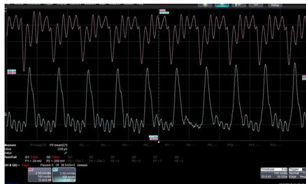
Figure 7: The time structure of MCP1 (upper signal) and photodiode (lower signal).
