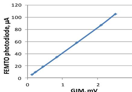
Figure 6: Dependence of XFEL Canberra PIPS diode current on gas ionisation monitor (GIM) signal at  $E_\gamma=9.66$  keV.
