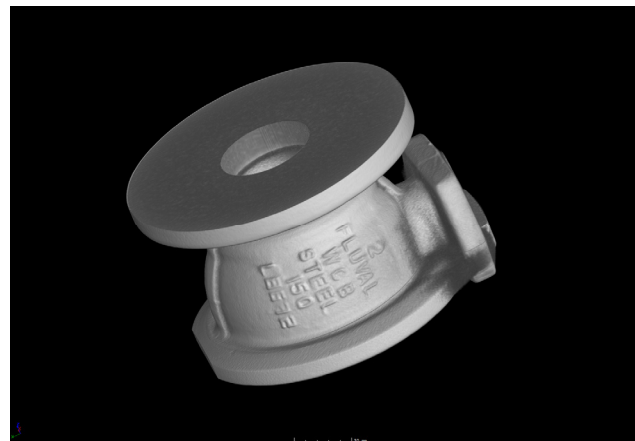
Figure 5: The reconstructed image of a valve.
