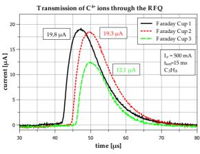
Figure 4: Transmission of a  $C^{4+}$  ion pulse from Faraday cup 1 (black solid line) to Faraday cup 2 (red dotted line) passing the RFQ to Faraday cup 3 (green dashed line).
