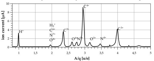
Figure 2: Ion spectrum with dominant  $C^{4+}$  ion peak measured at Faraday cup 1 at a pressure of  $8 \times 10^{-8}$  mbar, an ionisation time t<sub>ion</sub> of 15 ms, an electron beam current of 550 mA and an analyzing slit width of 10 mm. The fraction of  $C^{4+}$  ions results in 26 %.
