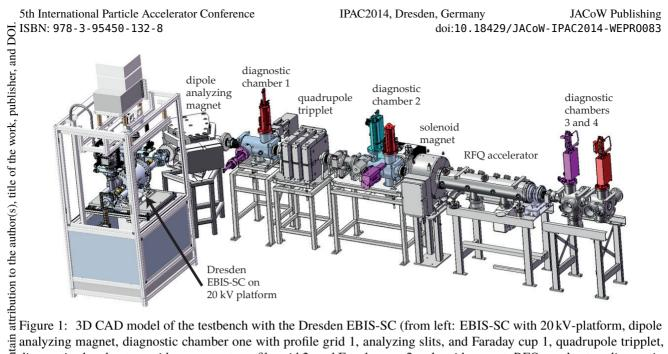
analyzing magnet, diagnostic chamber one with profile grid 1, analyzing slits, and Faraday cup 1, quadrupole tripplet, diagnostic chamber two with pepper pot, profile grid 2, and Faraday cup 2, solenoid magnet, RFQ accelerator, diagnostic chambers three, and four with a set of 3 phase probes, profile grid 3, and Faraday cup 3). The Faraday cups are colored in red, the grid profile monitors are colored in purple, and the pepper pot is colored in blue.
