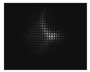
Figure 3: Pepper pot image captured from  $C^{4+}$  ions at the pulse ion current of 12 µA on the RFQ exit. The optical focus was set to the solenoid (Fig. 1), not to the pepper pot.
