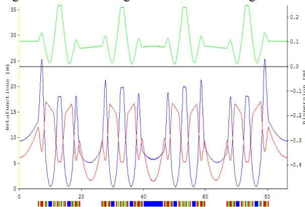
Figure 4: Beta function of MRW at short straight session of 1/6 superposition of TPS. we use left and right sides of three quadrupole magnets separately to simulate matching.
