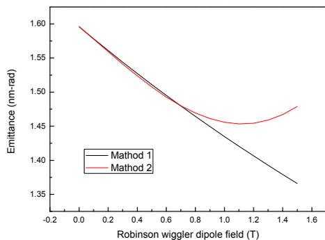
Figure 3: we consider the verified dipole magnetic field and find out the most effective magnetic field form Method2 formula. The value of magnetic field is about 1.1T.
