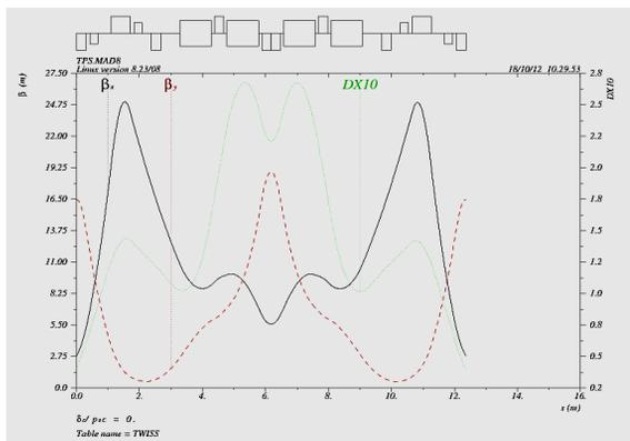
Figure 2: In order to improve damping partition number, we try to install three quadruples between each pole of Robinson wiggler. From matching result, the beam emittance reduce to 1.46 nm-rad, the reduction ratio is about 8.4%.
