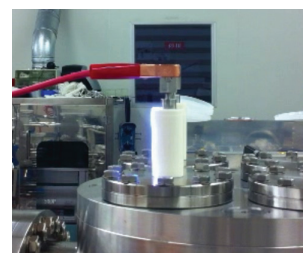
Figure 6: AC withstand voltage test of ceramic columns.
