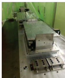
Figure 11: The adjustable plate, the Rapson-slide mechanism, stages for the kicker and pre-AC/AC septum were installed and aligned.
