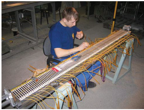
Figure 2 Half of the wiggler magnetic system under assembling procedure. The wiggler length is 1.8 m, period – 30 mm, magnetic field – 2.2T.
