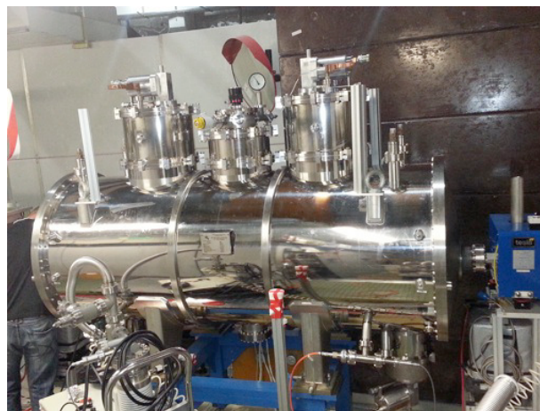
Figure 1: The refurbished superconducting wiggler installed in the Elettra storage ring.
