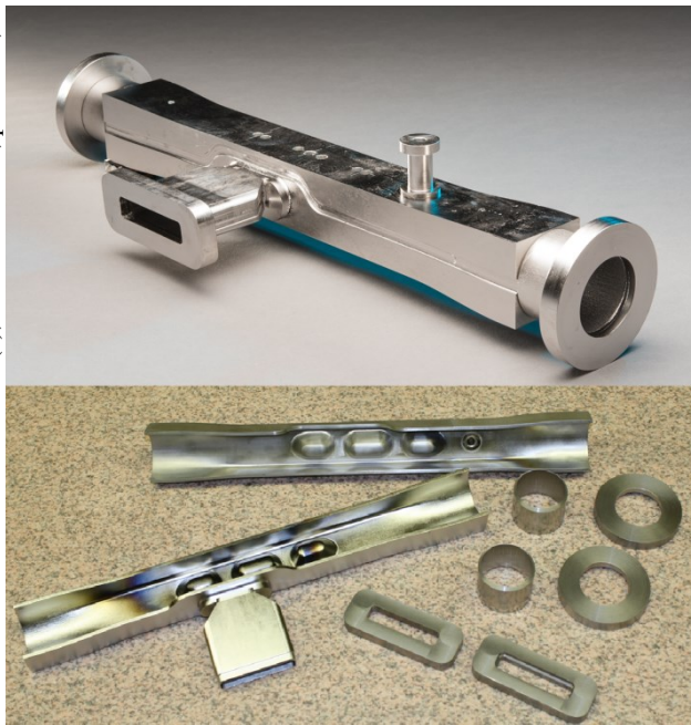
Figure 1: (Top) QMiR 21.75' Long, (Bottom) Niobium parts just before final welding.
