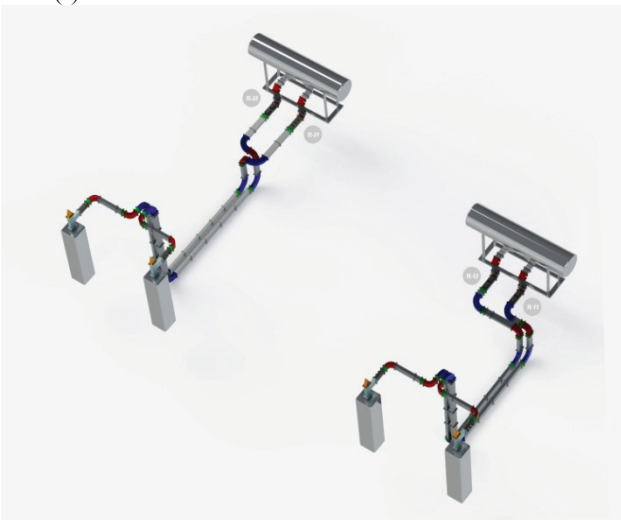
Figure 3: Schematic view of high power Transmission Line (II) of TARLA.
