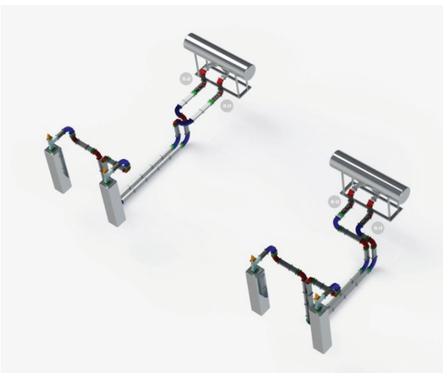
Figure 2: Schematic view of high power Transmission Line (I) of TARLA.
