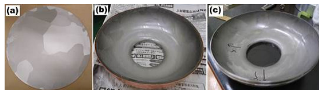
Figure 1: (a) LG-Nb disk supplied from Tokyo Denkai. (b) Half-cell with a copper shell. (c) Trimmed half-cell.
