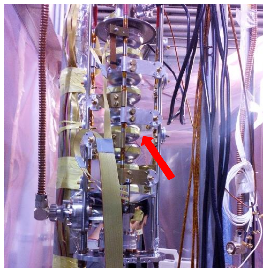
Figure 5: Fast thermometry sensors installed on the cavity together with OSTs.
