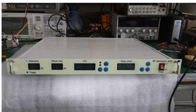
(a) Automatic frequency control (module)
