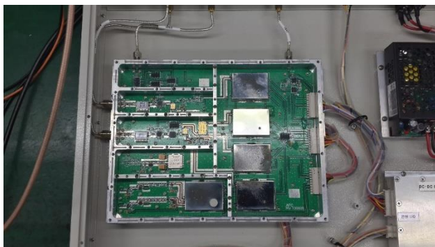
(b) Automatic frequency control module (inside)
