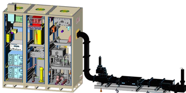
Figure 8: VIL410 cabinet layout and circulator.
