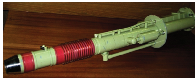
Figure 1: High-power klystron with magnetron gun.
