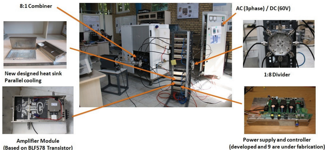
Figure 5: 4KW amplifier and its constructive components.
