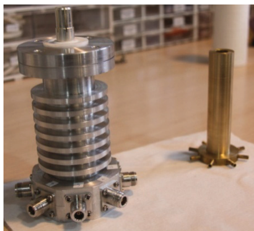
Figure 6: The radial coaxial combiner (4KW). Whole structure (left one) and inner conductor (left one).
