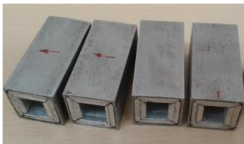
Figure 6: Assembled extraction magnets.
