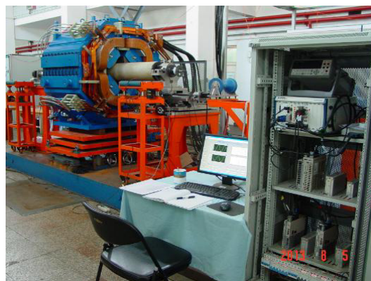
Figure 1: Quadrupole and Setup of the Rotating Coil.
