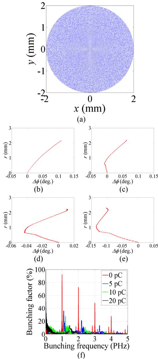
Figure 5: (a) Particle distribution of the electron bunch in the  $x-y$  plane at the cathode.  $r-\Delta\phi$  distributions of the electron-pulse trains with total charges of (b) 0, (c) 5, (d) 10 and (e) 20 pC at the accelerator exit. (f) Bunching factor spectra of the electron-pulse trains at the accelerator exit.
