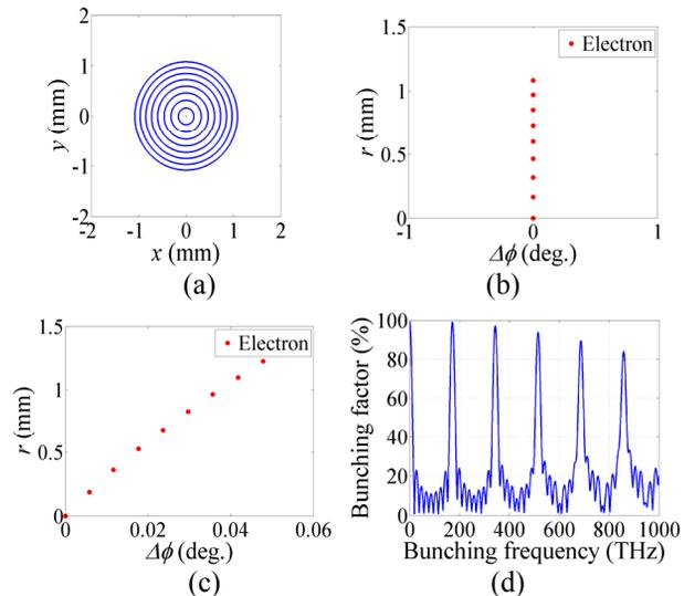
Figure 3: (a) Distribution of the electrons in the  $x-y$  plane at the cathode.  $r-\Delta\phi$  distributions of the electrons (b) at the cathode and (c) at the photoinjector exit. (d) Bunching factor spectrum of the electron-pulse train at the accelerator exit.
