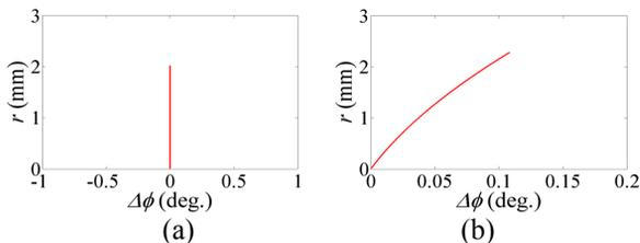
Figure 2:  $r-\Delta\phi$  distributions of the particles in an accelerated electron bunch (a) at the cathode and (b) at the exit of a typical S-band photoinjector. Results obtained from simulation in PARMELA.
