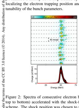
Figure 2: Spectra of consecutive electron bunches (from top to bottom) accelerated with the shock-front injection scheme. The shock position was chosen to select 50 MeV bunch energy. The average bunch charge was 90 pC, with little shot-to-shot fluctuations, as indicated in the line-out. Image taken from [12] with permission from APS.
