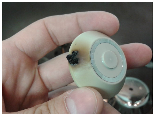
Figure 4: An insulator which was destroyed during the tests.
