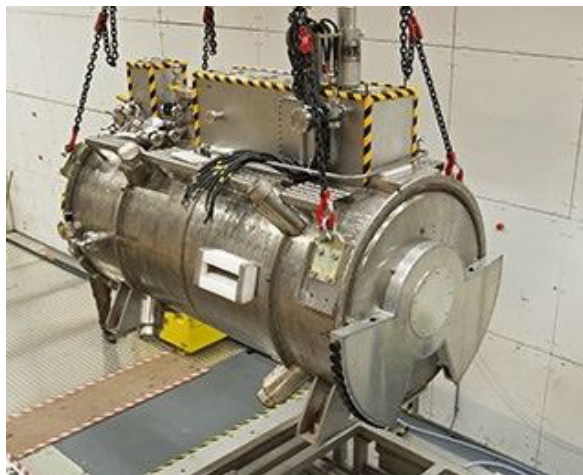
Figure 3: The first MICE spectrometer solenoid fitted with a fiber tracker is being moved to the MICE hall.
