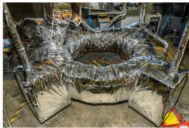
Figure 7: First CC cold mass at the Solenoid Test Facility at Fermilab after MLI rewrapping.
