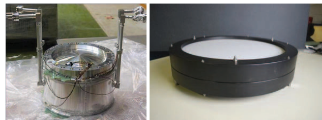
Figure 5: Liquid hydrogen (left) and lithium hydride (right) absorbers.
