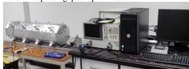
Figure 5: Experiment platform of the RFQ cold model.
