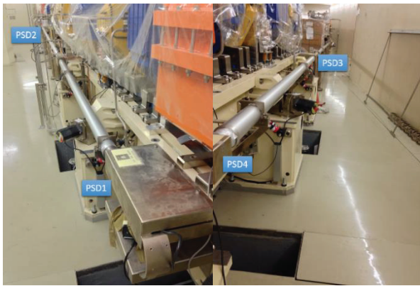
Figure 2: Four PSDs (PSD1, PSD2, PSD3 and PSD4) are installed beside girders respectively.
