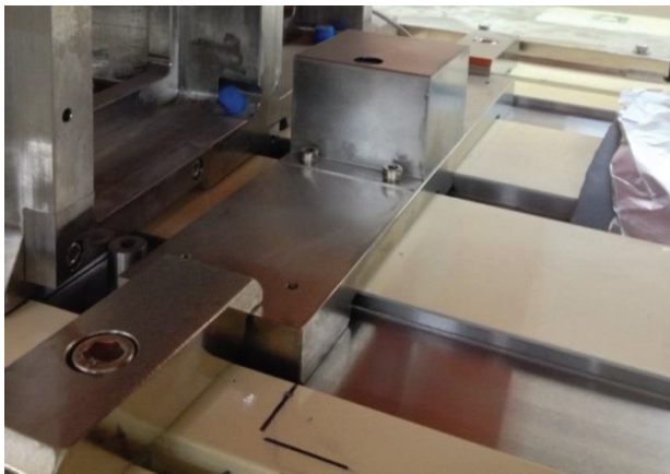
Figure 3: Precision inclination sensor is installed on each girder.
