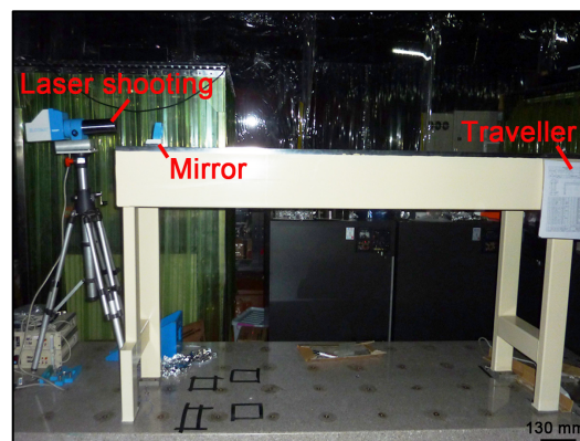
Figure 2: Measurement and erection of laser alignment tool.
