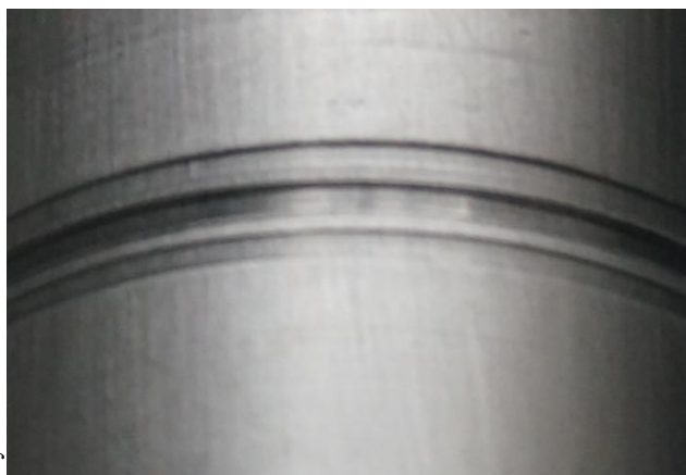
Figure 4: Roping at the shaft sleeve. The picture shows a close-up of a notch (1.5 mm width, 0.5 mm depth) on a stainless steel shaft sleeve (50 mm diameter).
