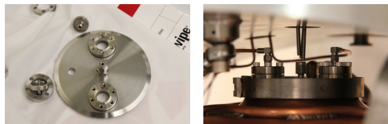
Figure 2: RF pickup probes installed through the top hat of the cavity. SMA connectors are used.
