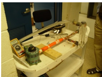
Figure 6: Mock-up of the central stem cooling circuit (above); testing the mock-up.
