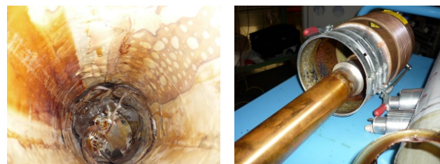
Figure 2: Klystron based transmitter ageing: damaged insulation of the linear HV transformer laminated core and burnt klystron output coaxial line.
