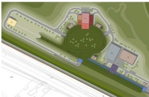
Figure 3: Tau/Charm complex including Main Rings, Injection complex and FEL facility (left). MR layout (right).
