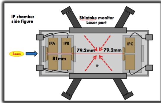
Figure 8: The distances between each low-Q IP-BPM.
