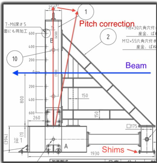
Figure 5: Pitch angle correction of IP-chamber.
