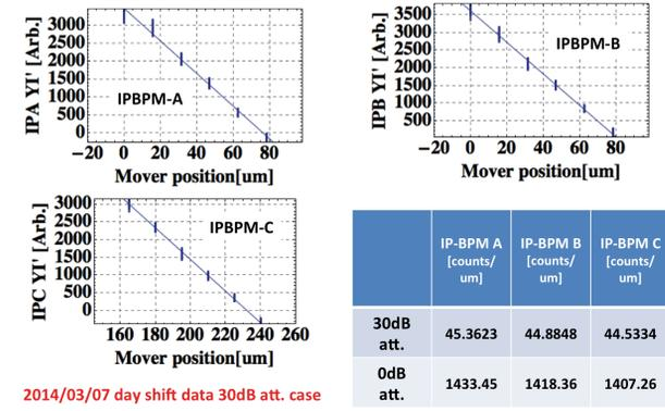
Figure 7: Low-Q IP-BPM calibration factor for 30dB attenuation.
