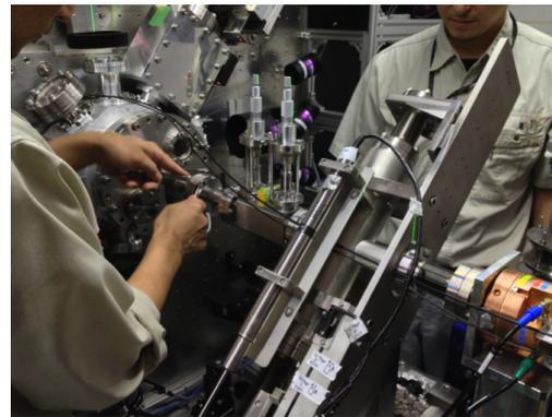
Figure 2: Installation of reference cavity BPM.
