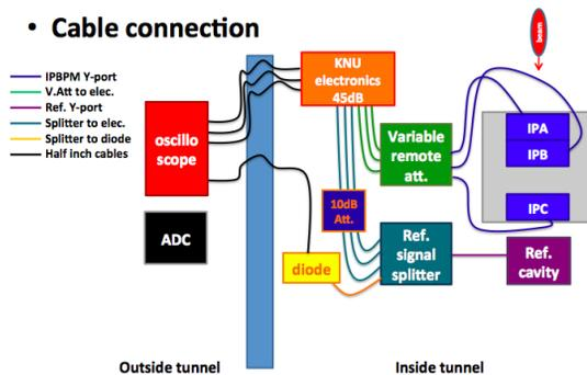
Figure 1: Low-Q IP-BPM cable connection scheme.
