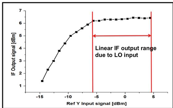
Figure 4: LO signal working range test of electronics.
