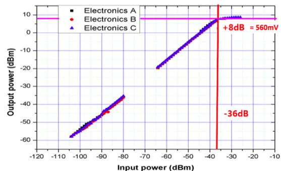
Figure 3: RF signal working range test of electronics.
