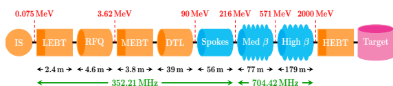
Figure 1: Schematic layout of the ESS Linac. Orange (normal temperature) and blue (superconducting) colors indicate a temperature of a section.
