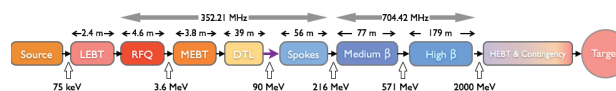
Figure 1: Block layout of the ESS baseline linac 2013, OptimusPlus (not to scale). Warm colored boxes represent the normal conducting components and cold color boxes the superconducting sections.
