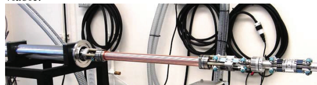
Figure 1: Photo of the magnetron assembly: 50-cm long cathode magnetron and spring loaded guide wheels. Leading edge guide wheels are inserted in a full-size RHIC tubing section.
