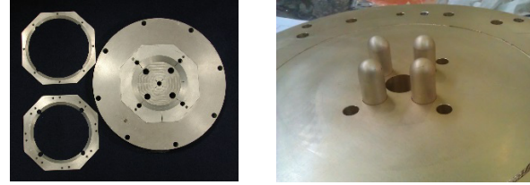
Figure 3: Example of tuning devices: adjustable thickness plates (left) and quadrupole rods set (right).
