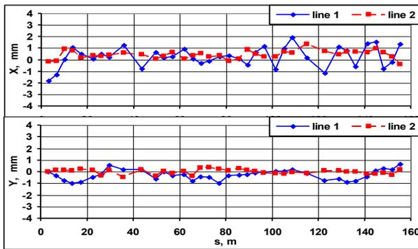
Figure 2: Horizontal and vertical orbit of beam at 200 MeV before (blue) and after (red) using the improved model.
