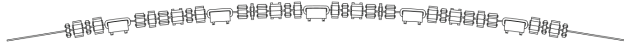
Figure 5: Magnets structure of a super period of the ILSF ring based on third option.
