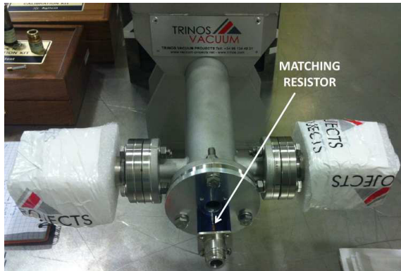
Figure 5: Resistor connected at both ends of the wire, in order to obtain one-way matching of the characteristic impedance of the line Z_{line} to the system impedance Z_0 .
