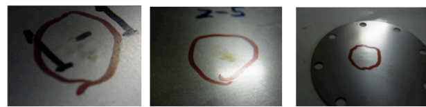
Figure 7: Thickness dependence of the damage in Ti plate.
