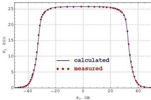
Figure 5: Field longitudinal distribution  $B_z(s)$  at 9.9 kA.
