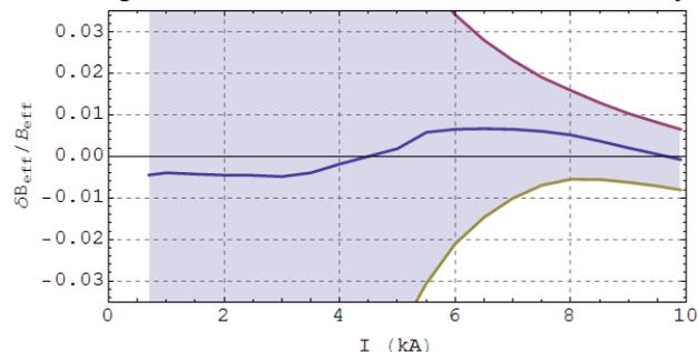
Figure 10: Difference in two type dipoles effective field.
