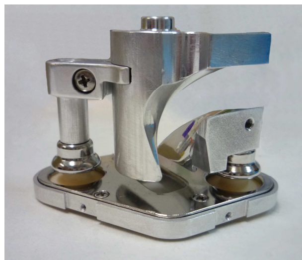
Figure 4: The electrodes of the spiral inflector.
